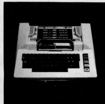
Atari 800 Console (with cover removed)
